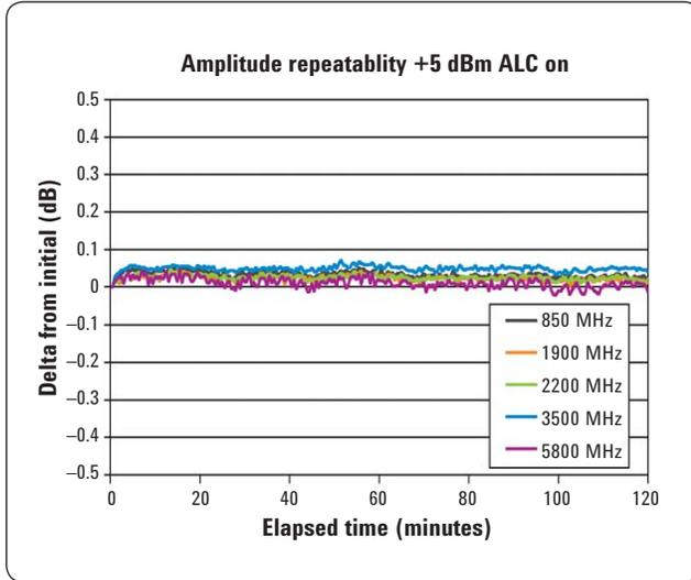
Repeatability measures the ability of the instrument to return to a given power setting after a random excursion to any other frequency and power setting. It should not be confused with absolute level accuracy.
